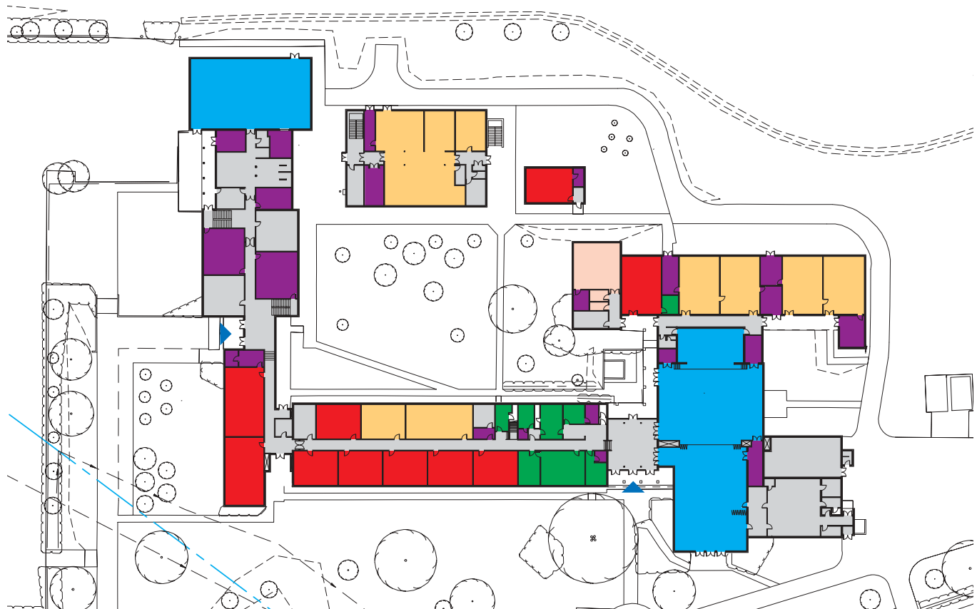
Site and ground floor plan (blue line shows route of main drains)
