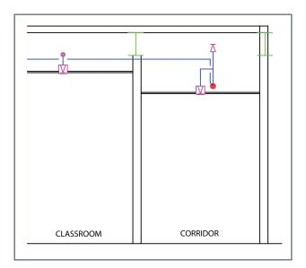
A side view of sprinklers and pipework in a classroom and corridor, section B-B.
