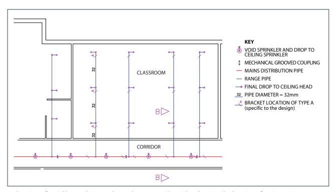
A plan view of sprinklers and pipework in a classroom and corridor, showing the location of section B-B
