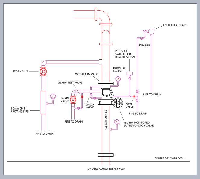
An example town main water supply and sprinkler valve arrangement
