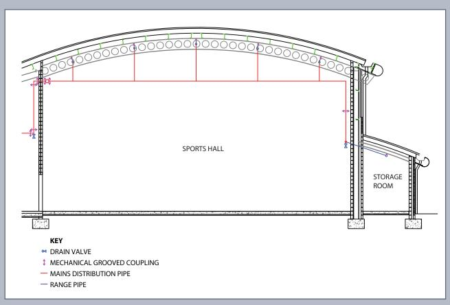
A side view of sprinklers and pipework in a sports hall and storage room
