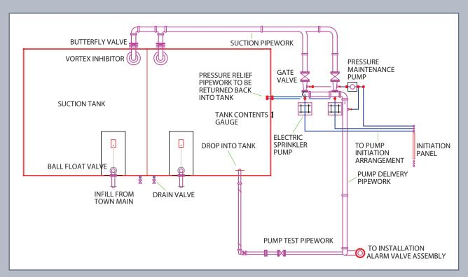
An example duplicate pump and tank water supply
