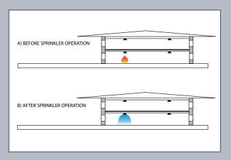
Schematic showing sprinkler head operating to control the fire
