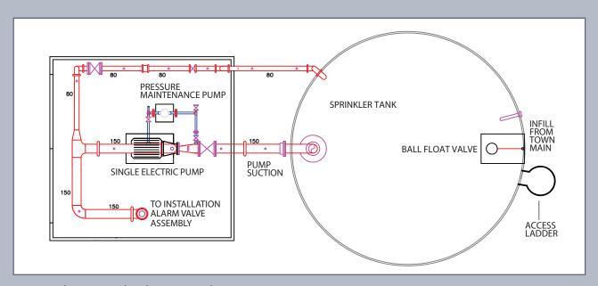
An example pump and tank water supply
