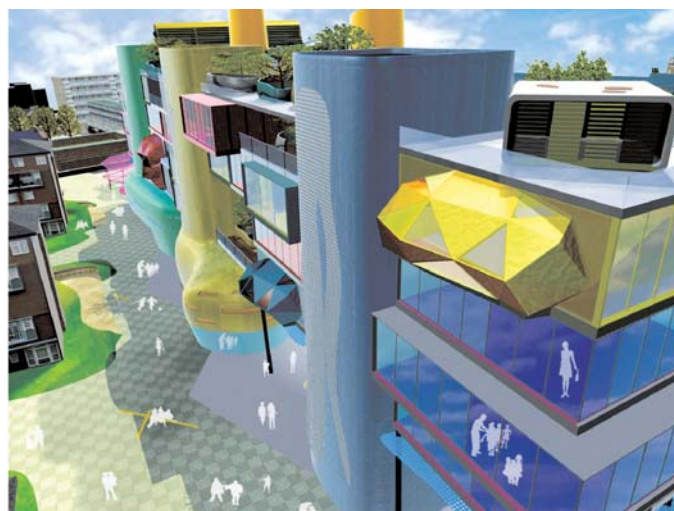
In the ‘test-bed’, different prefabricated practical learning spaces can be ‘plugged in’ between the stair towers, to suit the requirements of the school (model 4 design illustrated)
