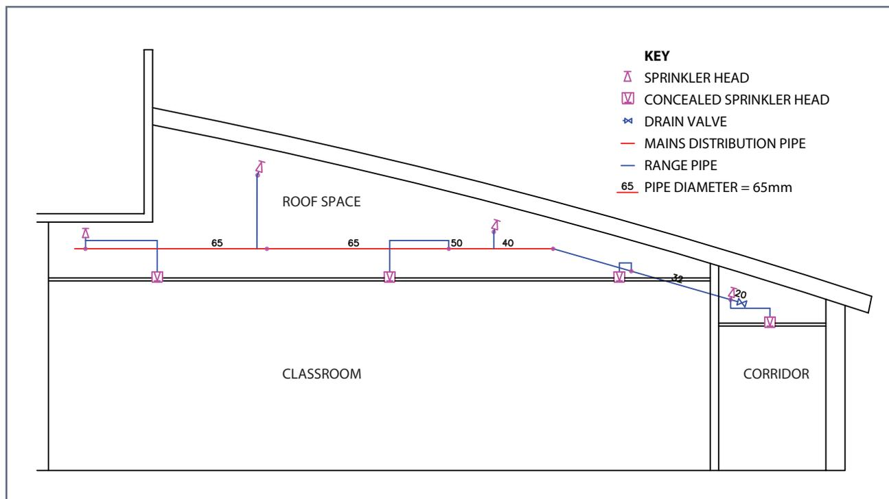
A side view of sprinklers and pipework in roof space, classroom and corridor
