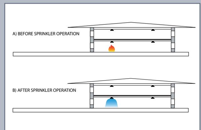
Schematic showing sprinkler head operating to control the fire
