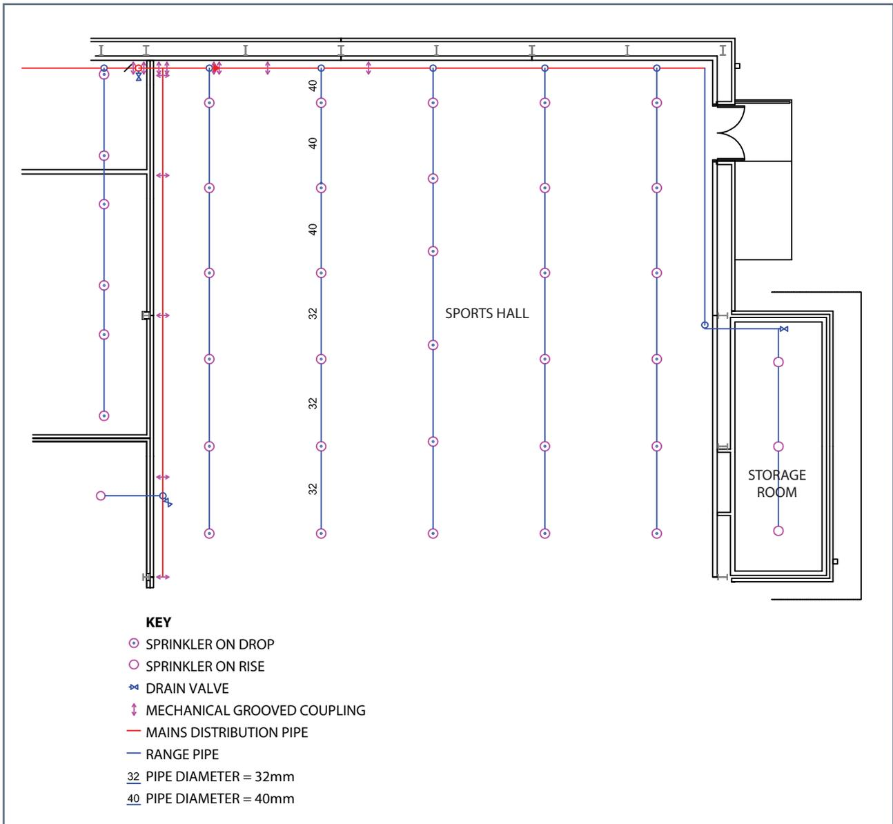
A plan view of sprinklers and pipework in a sports hall and storage room
