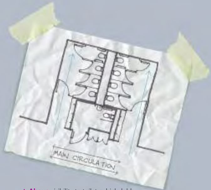
▲ Above visibility to toilet cubicle lobby
