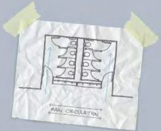
▲ Above visibility to toilet cubicle lobby
