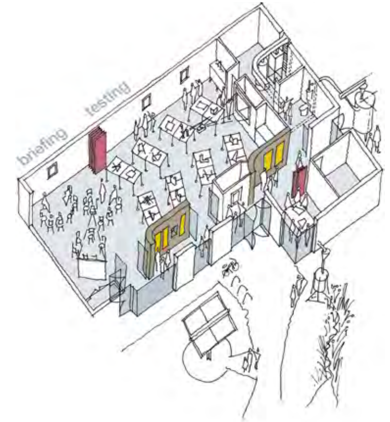
The main room is set up to learn about sustainable buildings with one zone for briefing and discussion and another for testing materials. Interactive display in the breakout area is visible on entry. Sustainability features are easily seen by those using the centre.
